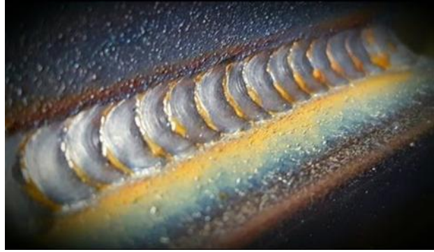
Figure 1 Straight bead weld considered between longitudinal bulb flat profiles and side shell
