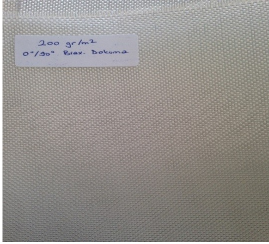
Şekil 5. 0°/90° Biaxial Cam Elyaf, 200 gr/m 2 .
