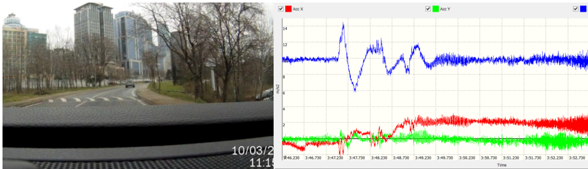
Figure 3: The Photograph and the accelerations of the 7 th Speed Bump.
