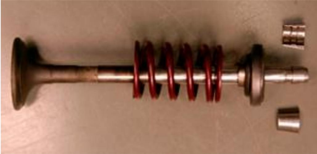
**Figure 3.** Valve and components.
