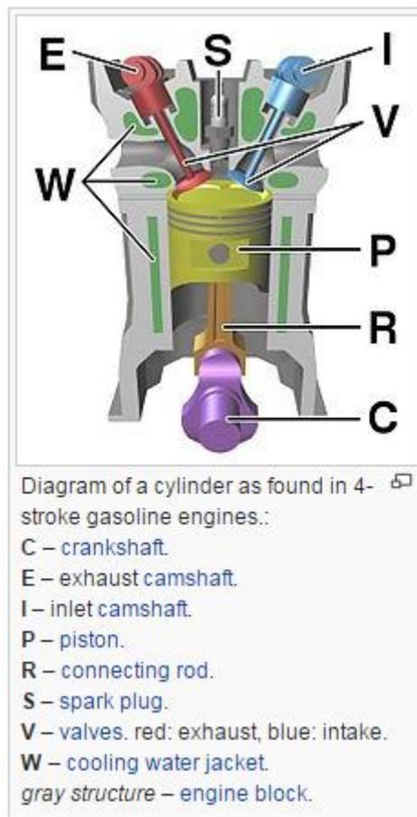
**Figure 1.** Diagram of a cylinder as found in 4-stroke gasoline engines.
