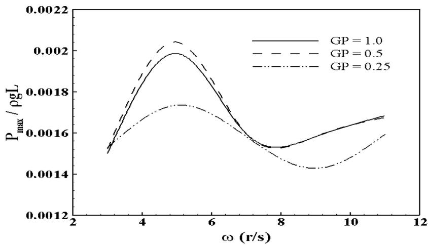
Fig. 12. Maximum pressures at T2.  $\theta_0 = 4^\circ$  ;  $h_p / h = 1/3$ .
