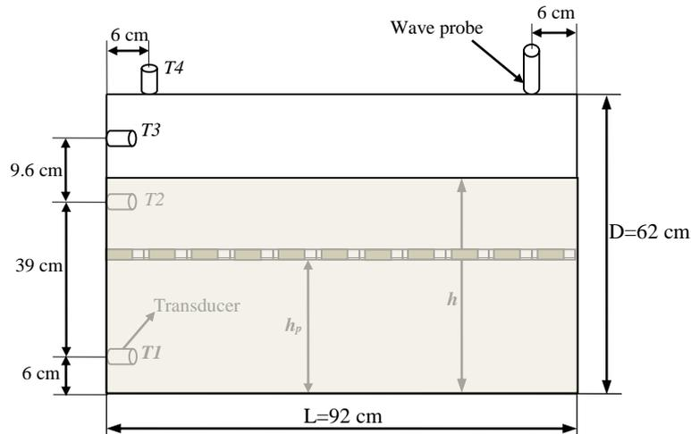
Fig. 1. Schematic diagram of the perforated plate configuration
