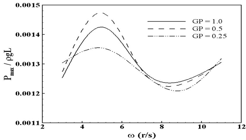
Fig. 14. Maximum pressures at T2.  $\theta_0 = 2^\circ$  ;  $h_p / h = 1/2$ .
