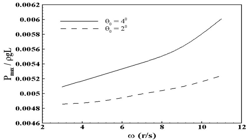
Fig. 2. Maximum pressures for an un-baffled tank at T1.
