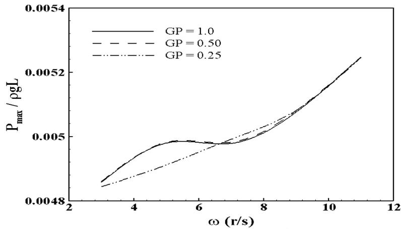
**Fig. 7.** Maximum pressures at T1.  $\theta_0 = 2^\circ$ ;  $h_P / h = 2/3$ .
