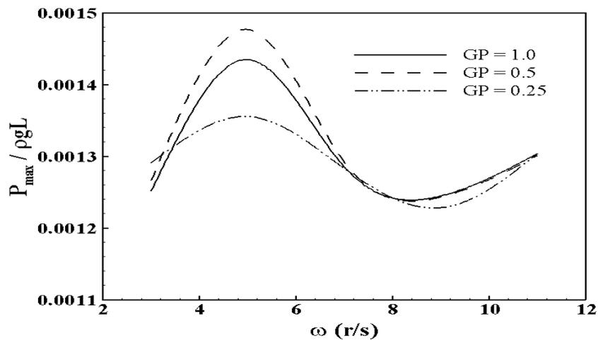
Fig. 15. Maximum pressures at T2.  $\theta_0 = 2^\circ$  ;  $h_p / h = 1/3$ .
