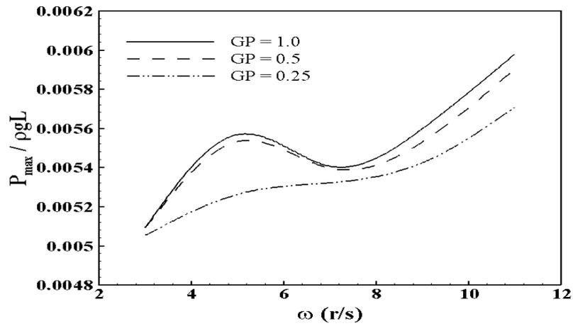
**Fig. 6.** Maximum pressures at T1.  $\theta_0 = 4^\circ$ ;  $h_P / h = 1/3$ .
