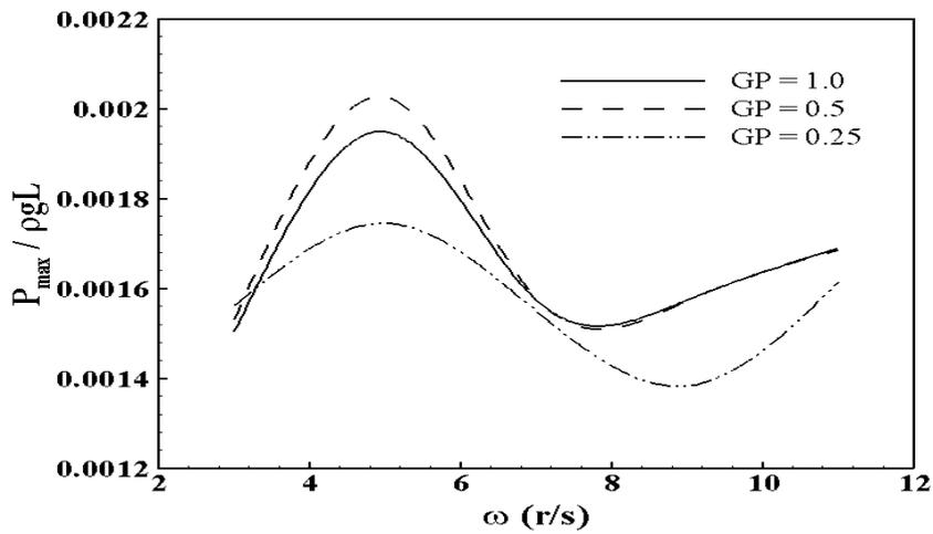
Fig. 11. Maximum pressures at T2.  $\theta_0 = 4^\circ$ ;  $h_p / h = 1/2$ .
