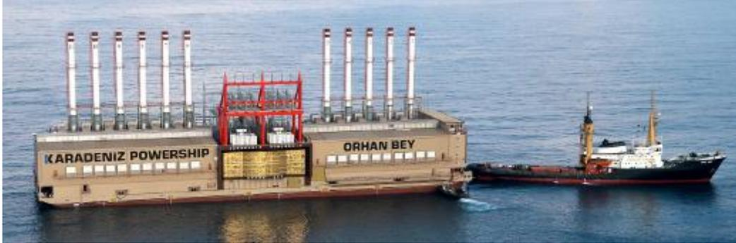
**Figure 2.** None propelled power plant
