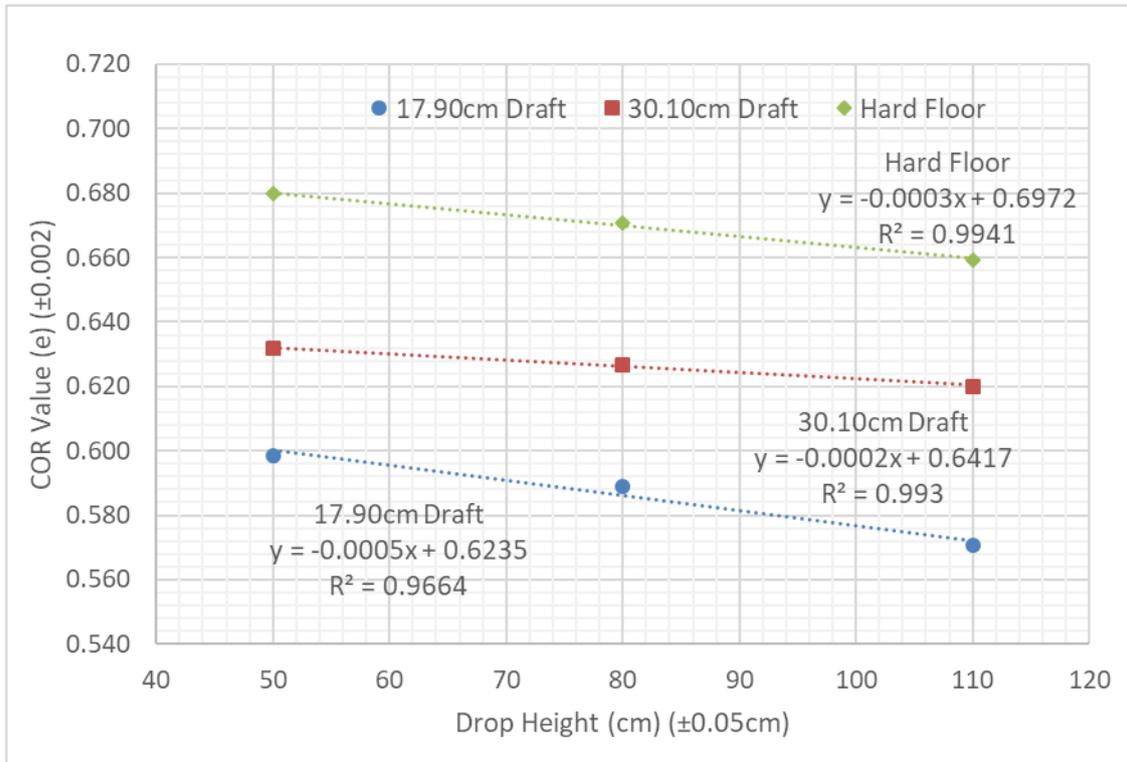
Figure 8: COR Value Versus Drop Height of Plastic Ball
