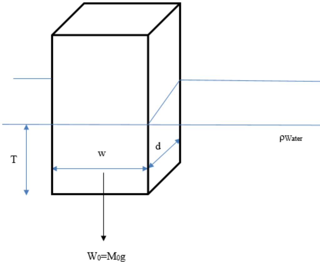
**Figure 1:** Rectangular Prism Floating in Water
