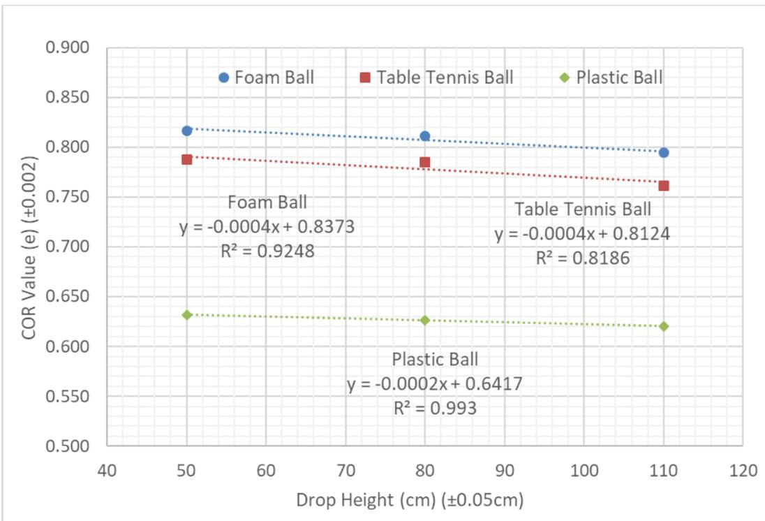
Figure 10: COR Values of All Balls, Submerged in Water, 30.10cm Draft
