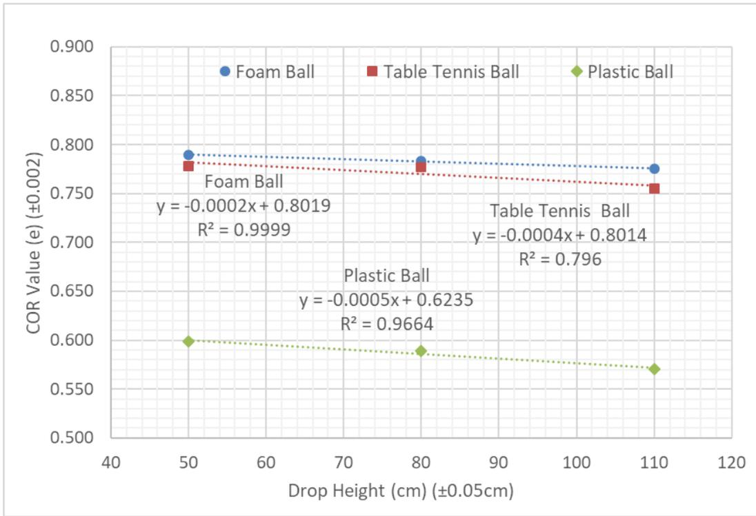
Figure 9: COR Values of All Balls, Submerged in Water, 17.90cm Draft
