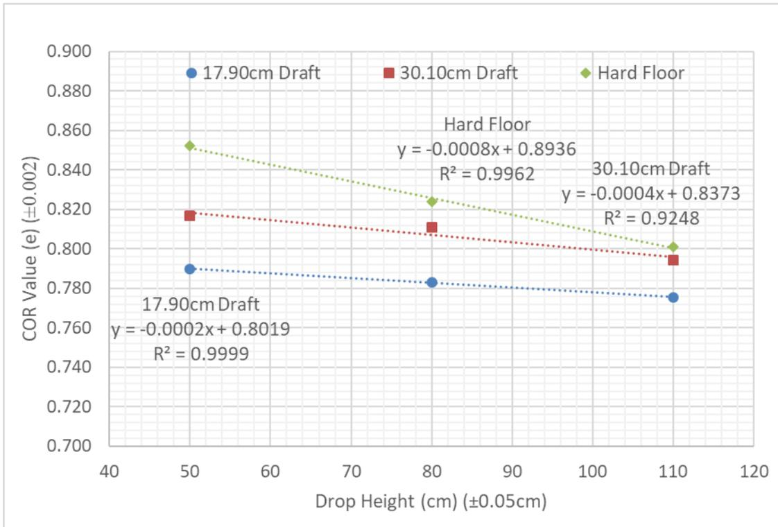
Figure 6: COR Value Versus Drop Height of Foam Ball
