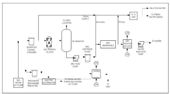
Figure 3.6 Water Injection System.
