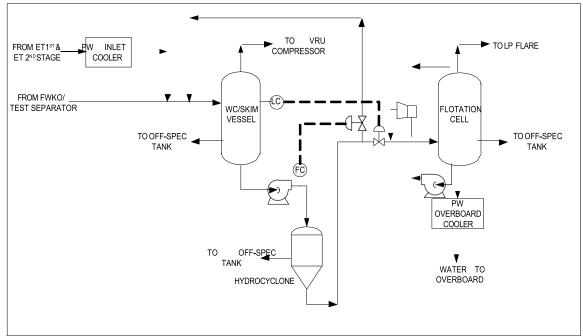
Figure 3.5 Produced Water System.
