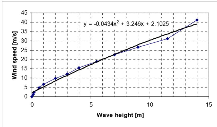
Figure 2. Wind speed vs. significant wave height from the Beaufort relationship. Solid line is the fitted 2<sup>nd</sup> order curve
